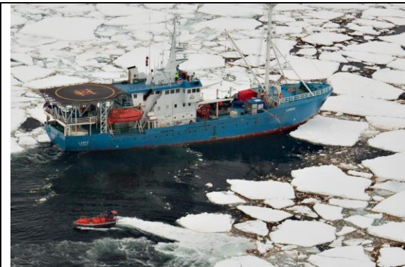
Fig. 14: RV Lance research vessel testing dispersant effectiveness in pack ice by directing mixing energy to the oil (lower right) with the MOB boat.
