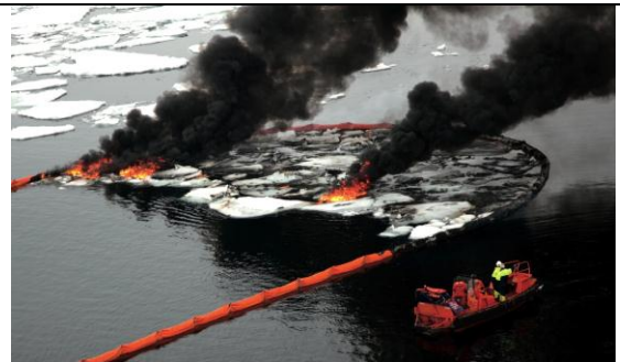
Fig. 15: Burning oil mixed with ice cakes and pieces collected within a fire resistant boom. Photos: SINTEF Oil in Ice JIP
