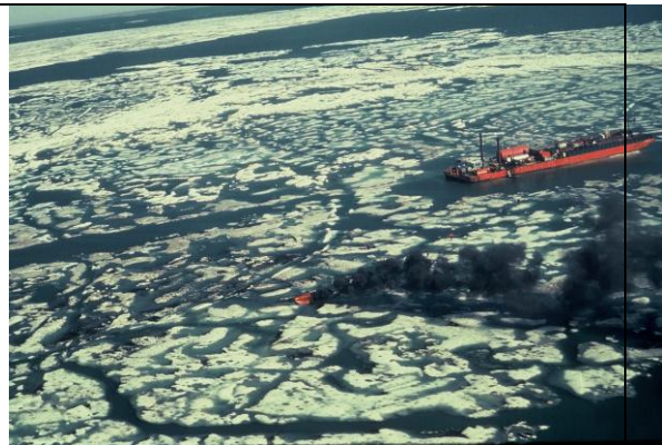
Fig. 5: Burning oil present on surface melt pools at McKinley Bay, NWT. July 4 1980, immediately prior to break-up. Photo: D. Dickins
