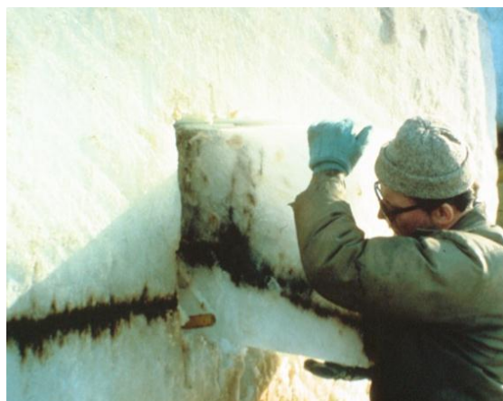
Fig. 6: Oil encapsulated in ice during an experimental spill in Alaska. Photo: A. Allen
