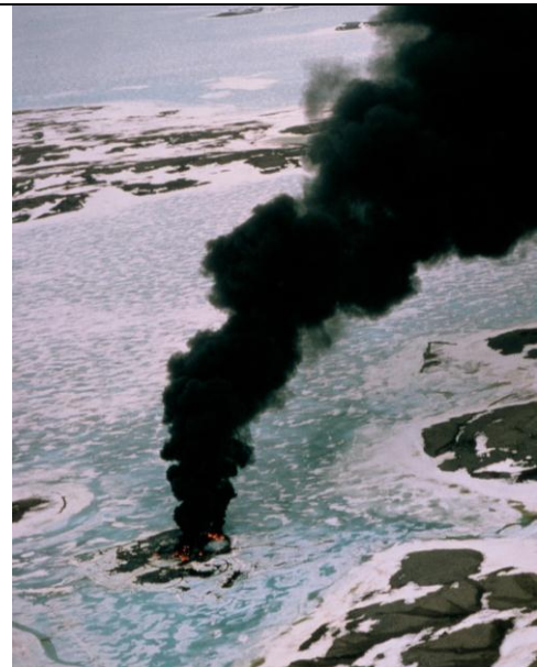
Fig. 3: First large-scale experimental burn of oil on ice in the Arctic, June 1975 at Balaena Bay. At the time of this photo, over 200 barrels of crude oil were burning with over 90% being consumed in 20 minutes.
