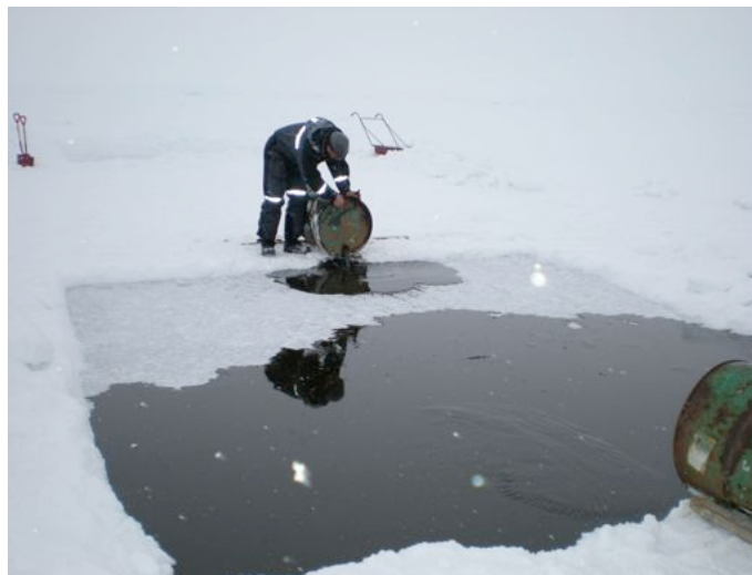
Figure 2. Photograph of Sintef personnel pouring oil into the spill containment area for the oil-under-snow field experiment.
