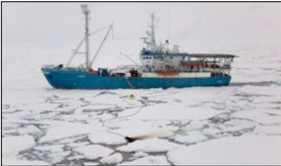
Figure 12. P1#2, 7 m 3 oil release May 15 at 0854. The oil is being pumped through the hose lying on the ice surface. Photo: Jan Nilsen.
