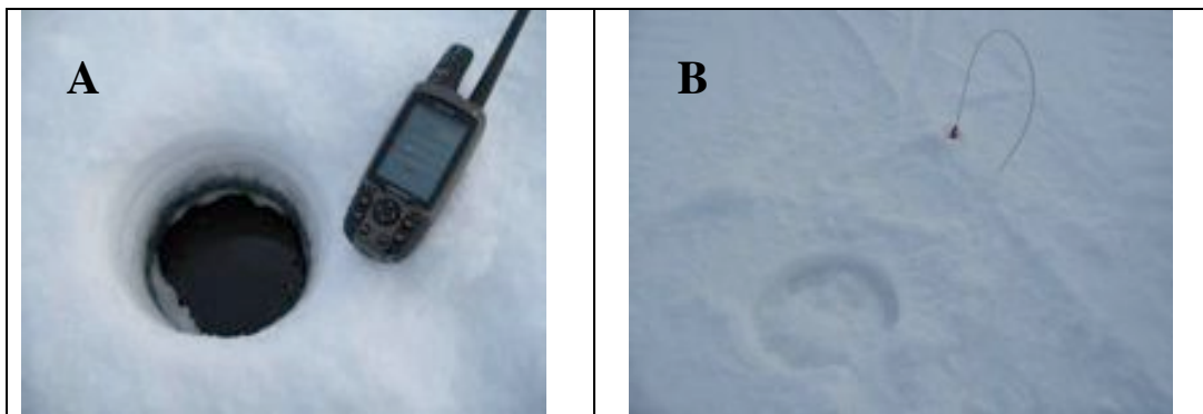
Figure 8. Small training oil spills used for the field training. A: 400 ml of weathered Troll crude (200°C+) in a 30cm hole in the first year ice. B: The hole covered with snow and ice chips.
